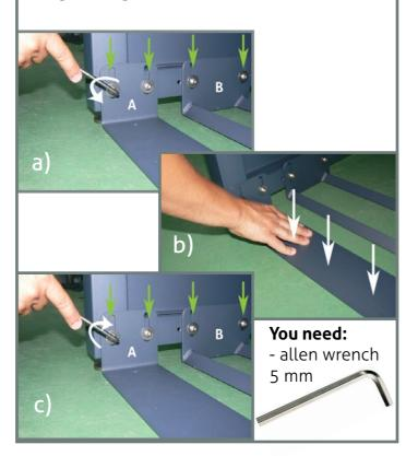
**5.** Tip: the wheel stabilizer is set to the middle position by default. If necessary, you can move the stabilizer and attach it forwards or backwards.
