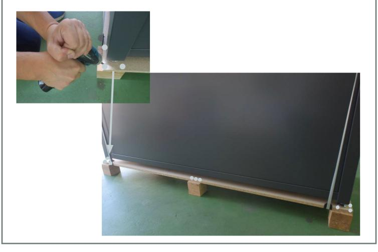
**2.2.** Carefully tilt the entire waste enclosure with the pallet forward to remove the carrying blocks with your foot. When all the blocks are removed, carefully let the waste enclosure go back so that the panel sits firmly on the ground.
